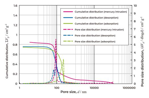
Particle size distribution determined by mercury intrusion method and BJH method (BELSORP MINI X)
