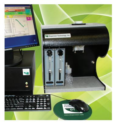
**Model DT-100 has a unique Acoustic sensor** for characterizing *particle size distribution* by measuring ultrasound attenuation at set of frequencies from 1 to 100 MHz, as well as sound speed. This method can be referred to as *"ultrasound scattering"*.
